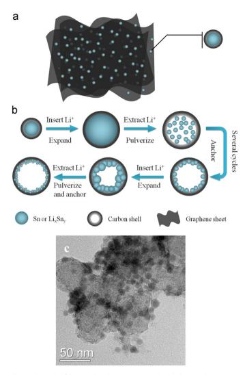
**Fig. 5.** Schematic of the Sn@C/graphene nanocomposite (a), the particle expansion and pulverization (b) and the TEM image of the material after being cycled (c). Pulverized Sn particles anchored on the carbon can be observed.
