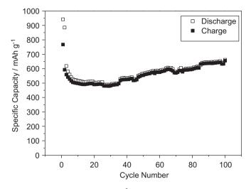
**Fig. 4.** Cycle performance at 100 mA  $g^{-1}$  of the Sn@C/graphene nanocomposite.
