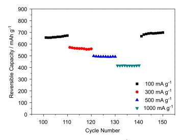
Fig. 6. Cycle performance after 100 cycles at 100 mA  $\rm g^{-1}$  of the Sn@C/graphene nanocomposite.
