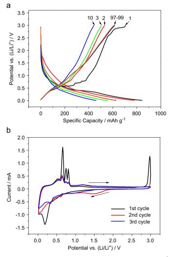
**Fig. 3.** Discharge–charge curves (a) at the specific current of  $100 \text{ mA g}^{-1}$  (the cycle numbers were labeled with arrows) and the cyclic voltammograms (CVs) curves (b) of the Sn@C/graphene nanocomposite.
