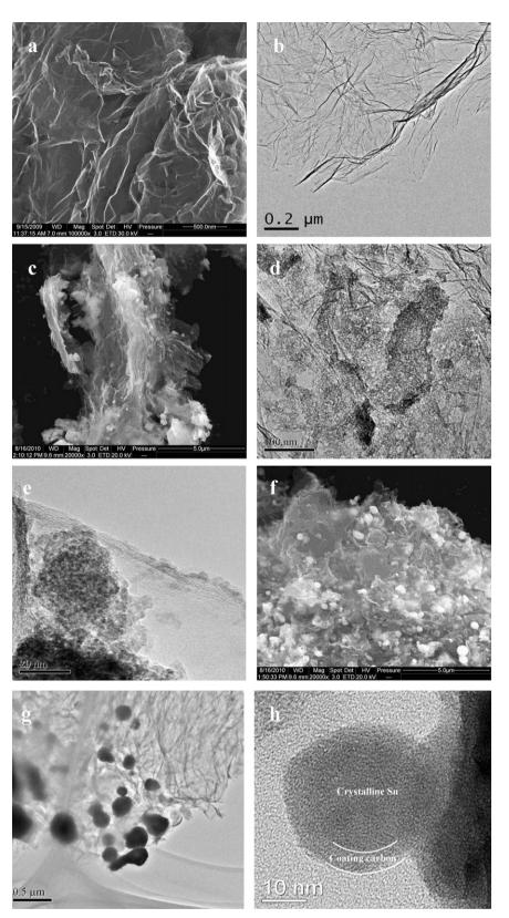
Fig. 2. SEM and TEM images of graphene (a and b), SnO<sub>2</sub>/graphene (c-f) and Sn@C/graphene (f-h). The coating carbon and crystalline Sn are marked in (h).
